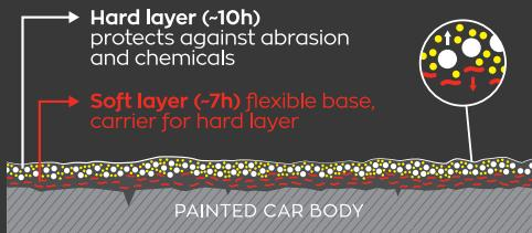
Key to Crystal Serum Ultra's performance gain is the introduction of a revolutionary new 7nm nanoparticle alongside an existing 20nm nanoparticle, and increasing the ratio of crosslinkers, which reinforce and thicken the top layer.
